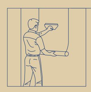
Smoothen out all the bubbles using Smoother or Roller as required.
